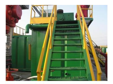
TANK SIDE END WALLS AND PARTITIONS SHOULD BE MADE BY ST-52, 5/16" PLATE.
